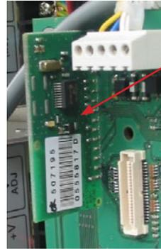
Tarjeta receptora radio HF
